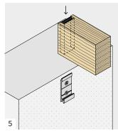
Hook the beam fitting it from the top to the bottom.
