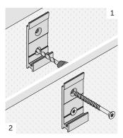
Place the connector on concrete and fasten the anchors according to the installation instructions.
