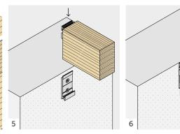
Hook the beam fitting it from the top to the bottom.
