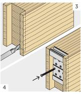
Perform full grooving on the secondary beam. Position the connector and fasten all screws.
