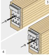
Place the connector on the wooden beam and fasten the first screws. When using LOCK STOP (optional) position LOCK STOP and fasten the remaining screws.
